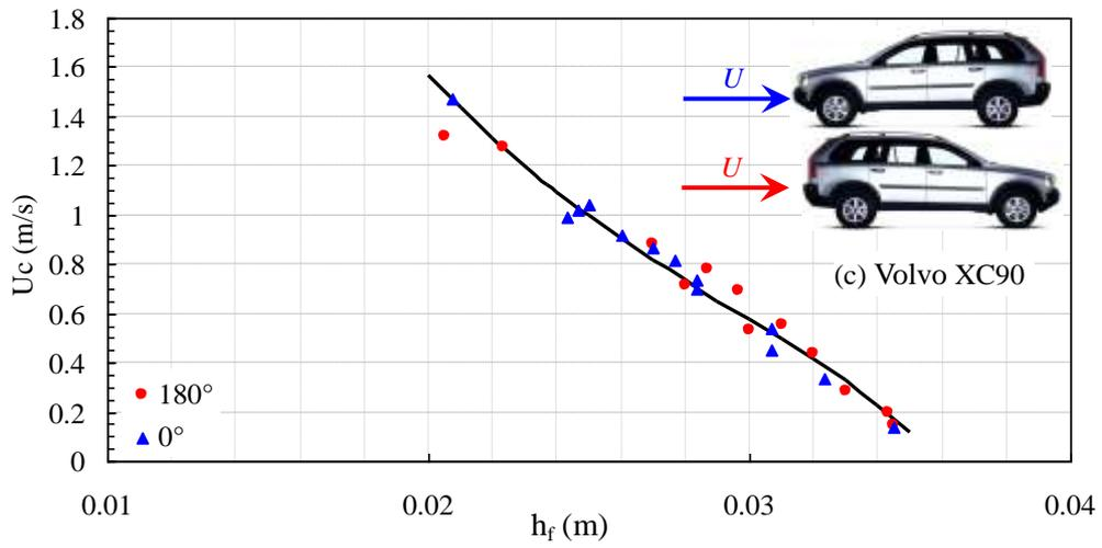
Depth-incident velocity relationships for partially submerged model vehicles
