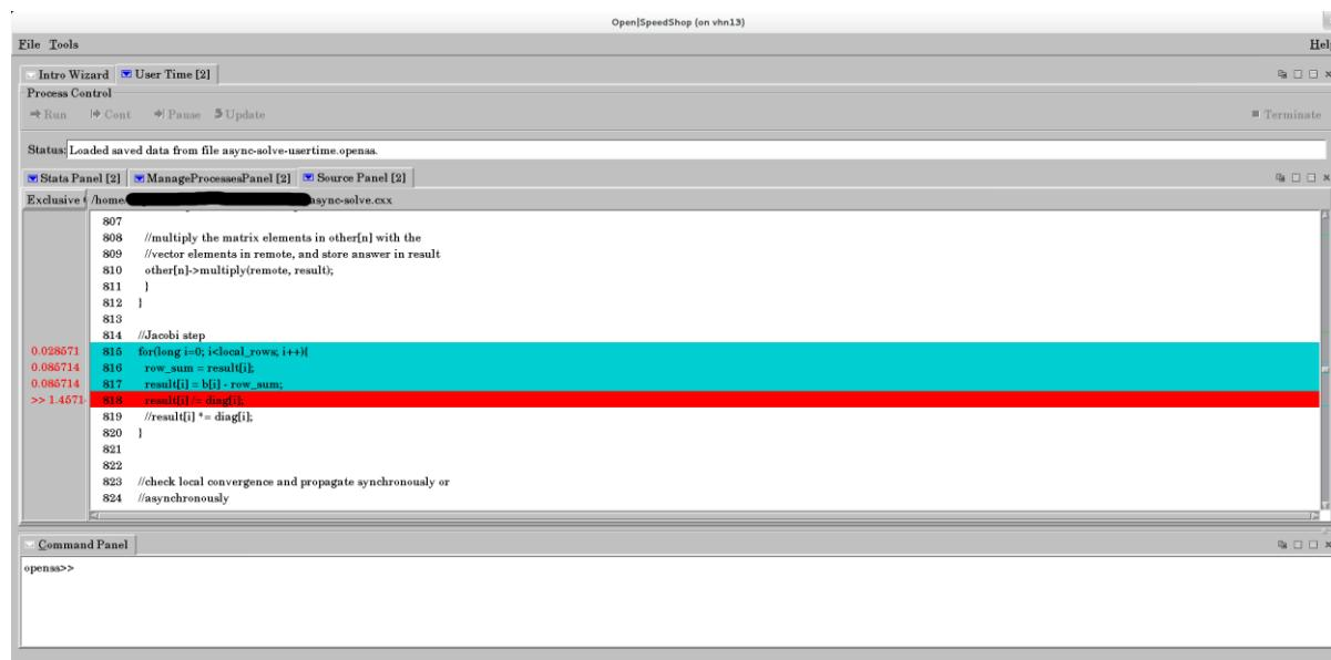
Here, we selected the top line on the default display, and in the resulting source code display this line (818) is highlighted in red as it was the line on which the code spent the highest proportion of time.
